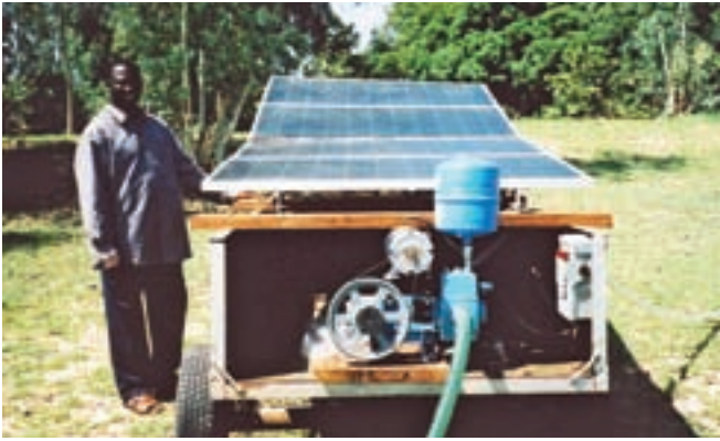
This PV array provides energy for a mobile solar irrigation pump. The cart, moved from field to field by two cattle, enables farmers to irrigate their crops during the dry season, providing food and income for their families.
